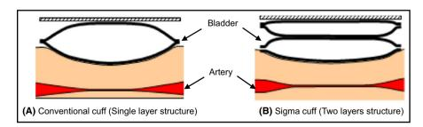
**FIGURE 2** Cross-sectional diagram of a conventional cuff with a single-layer bladder (A) and the Sigma cuff with a two-layer bladder (B). In the case of the Sigma cuff, the flat section length of arterial occlusion is greater than in the conventional cuff due to the two-layer bladder structure, which would lead to more adequate sensing of the cuff pressure pulse wave
